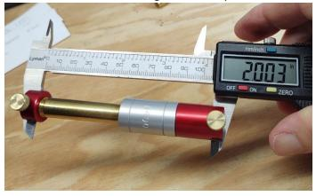
Shoulder measurement using the Hornady Lock-N-Load Headspace Gauge – Fired from T/C Compass II
